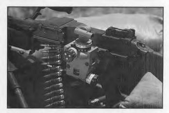
Sophisticated H-019 long-range dial sight can be mounted to the left side of the SS-77 receiver body for indirect fire from defilade along fixed lines.
